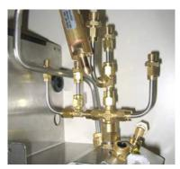
Boiler subassembly pre-fabricated by Serto, mounted and installed by customer.
