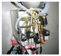
Boiler unit in the coffee machine, Serto unions join the media-conveying lines with the espresso module.
