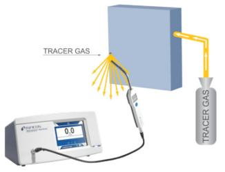
This method and the tracer gases will be explained more in detail in Section 3.
