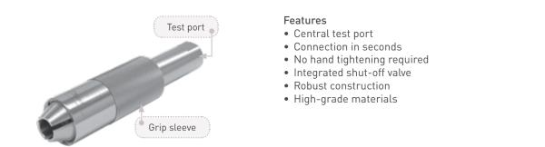
The WEH<sup>®</sup> Connector type TW711 has been specifically developed to connect fuel lines for engine hot testing. The design of the connector is best suited for narrow spaces and meets the demand of such applications. Type TW711 is equipped with a central flow and test port for ease of use. No need for time-consuming and tedious hand threading, thus saving costs and repetitive strain injury.
