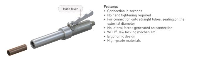
The WEH<sup>®</sup> TW141L Quick Connector has been developed for difficult to access test pieces. The extended jaws allow connection to difficult to reach tubes in narrow spaces - heat exchangers are a typical example. The design ensures that disconnection is not possible whilst still under pressure.
