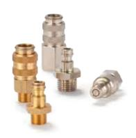
Mini industrial coupling with the world's most popular profile in this nominal diameter. Above average flow performance for liquid and gaseous media. It also uses an additional safety locking system. This prevents unintentional disconnection. When being disconnected, the plug must first be pushed further into the coupling before it can be disconnected.
