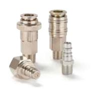
Safety coupling with UltaFlo-Valve for optimum flow and low pressure drop. The series stands out for its robust design (steel sleeve) and long service life even with the harshest use. Additional safety locking system. This safety lock prevents unintentional disconnection. To disconnect, the plug must first be pushed further into the coupling before it can be unlocked. The brass version has been developed specifically for use with water in the pressure range up to 35 bar.
