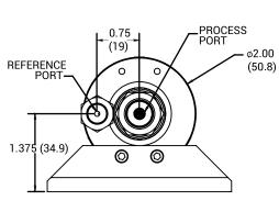
FITTING CODE "FF" WITH BAYONET CONNECTOR "B3"
