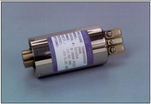
Setra Systems Model 280E/C280E pressure transducers are intended for low to high pressure measurements of gases or liquids in applications requiring rugged packaging, high performance and affordability. The 17-4 PH stainless steel capacitance sensing element, coupled with an IC-based circuit, assures excellent accuracy and long term stability.
