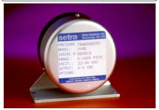
etra Systems Model 204D pressure transducer is intended for accurate differential pressure measurement of gas or liquid media compatible with 17-4PH stainless steel. The high level output signal and excellent stability, combined with fast dynamic response, make this unit ideal for industrial, laboratory, and aerospace applications requiring the highest accuracy. The 204D is thermally compensated for both zero and span shifts due to environmental temperature variations.
