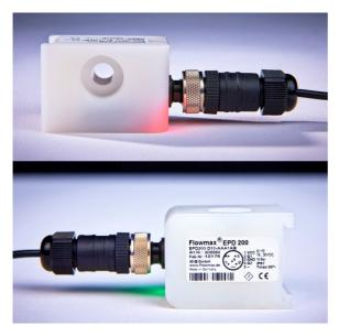
Flowmax EPD 200 is an empty pipe detection for use in conductive and nonconductive liquids. It is suitable as a pump protection against dry running, as a signal transmitter for 3way-valves for switching barrels, as liquids watchman or limit
