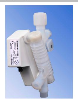
Flowmax 400i is a flow meter calculating the volume flow of liquids. Based on the ultrasonic technology Flowmax is able to measure conductive and non-conductive liquids contactfree. Flowmax has no moving parts and is absolutely free of wear. The design of the pipe minimizes dead space over the whole geometry.
