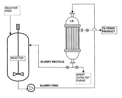
FIGURE 3: HyPulse LSM Filter For Integrated Closed-Loop Catalyst Recycle
